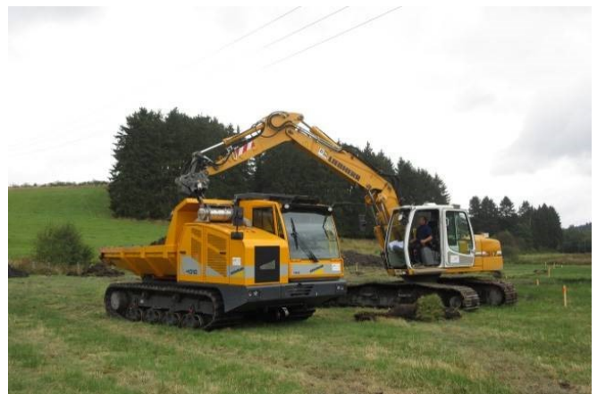
A dumper on chains reduces compaction of the soil without having to set up a construction road.
