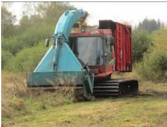
Figure 23. PistenBully converted into a mower with collection container
